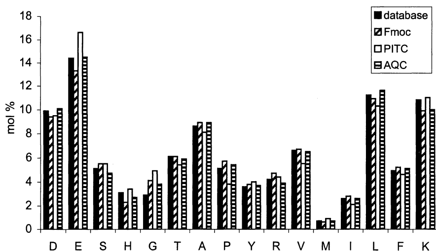
Fig. 7.3. Amino acid analysis of 1 \mu g (15 pmol) of PVDF-bound bovine serum albumin using three different derivatization chemistries. See Table 7.2 for a numerical presentation of this data
